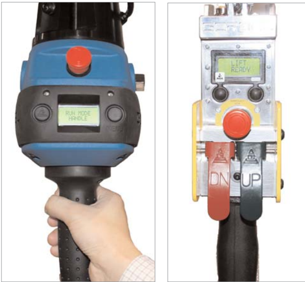
The LCD screens on the new standard handle (left) and pendant handle (right) communicate valuable information to both operators and to maintenance personnel.
